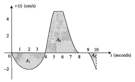
The graph above represents the velocity v of the cutting head of a computer controlled milling machine. Positive values of v represent movement to the right.
